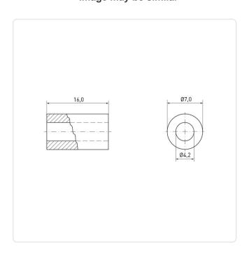
Finish: Plain For Thread Size: M4 Inner Diameter [mm]: 4.2 Length [mm]: 16
