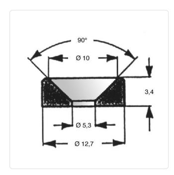
Color: White For Thread Size: M5 Height [mm]: 3.4 Inner Diameter [mm]: 5.3 Material: PA 6 Material Group: Plastic Outer Diameter [mm]: 12.7 Weight: 0.32g
