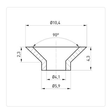
Inner Diameter [mm]: 4.1 Lug Diameter [mm]: 5.9 Material: PA 6 Material Group: Plastic
