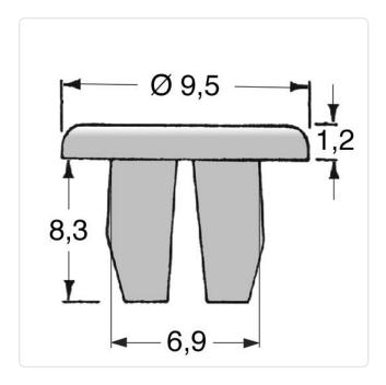
AF / OD [mm]: 9.3 Color: Natural Head Height [mm]: 8.8 Length [mm]: Material: PA 6.6 Material Group: Plastic Panel Cutout [mm]: 7.2x7.2 Panel Thickness [mm]: 0,8-4,0 Thread Diameter [mm]: Ø 4.2 Weight: 0.41g
