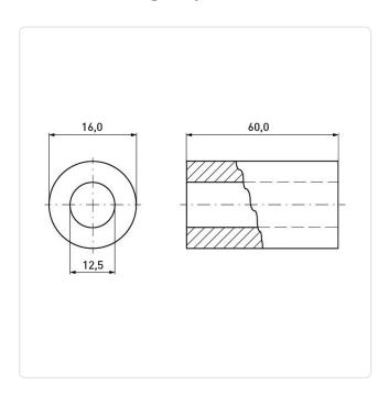
Color: Black Flammability Class: UL94-HB For Thread Size: M12 Inner Diameter [mm]: 12.5
