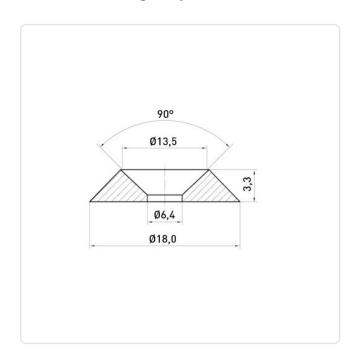
Finish: Plain For Thread Size: M6 Height [mm]: 3.3 Inner Diameter [mm]: 6.4
