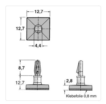
Color: Natural Flammability Class: UL94-V2 Length [mm]: 12.7 Material: PA 6.6 PCB Hole Ø [mm]: 3.2 PCB Thickness [mm]: 1,6 Weight: 0.62g
