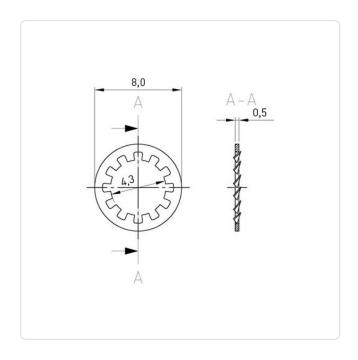
DIN/ISO: **DIN6797I** Finish: Plain For Thread Size: M4 0.5 Height [mm]: Inner Diameter [mm]: 4.3
