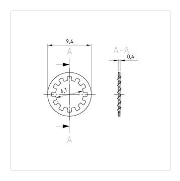
Finish: Plain For Thread Size: M6 Height [mm]: 0.4 Inner Diameter [mm]: 6.1
