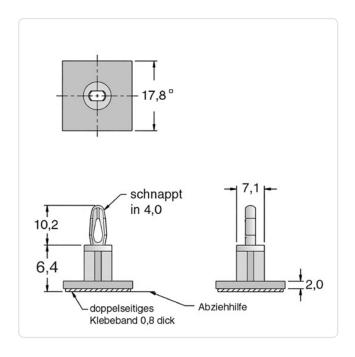
Color: Natural Flammability Class: UL94-V2 Length [mm]: 6.4 Material: PA 6.6 PCB Hole Ø [mm]: PCB Thickness [mm]: 1,6 Weight: 0.97g
