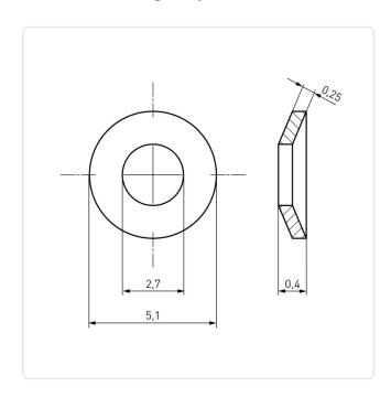
Finish: Plain For Thread Size: M2.5 Height [mm]: 0.25 Inner Diameter [mm]: 2.7
