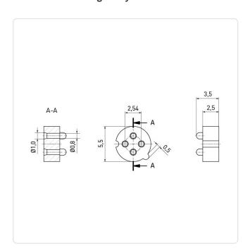
Length [mm]: 3.5 Material: PA 6.0 Model: TO-18 Outer Diameter [mm]: 5.5 Weight: 0.08g
