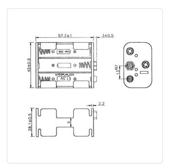
Battery Type: AA-Mignon Flammability Class: UL94-V0 Length [mm]: 77.06 Material: Plastic
