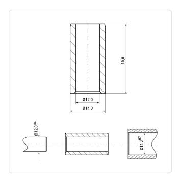
Color: Natural Flammability Class: UL94-V2 Inner Diameter [mm]: 12 Length [mm]: 10 PA 6.0 Material: Material Group: Kunststoff
