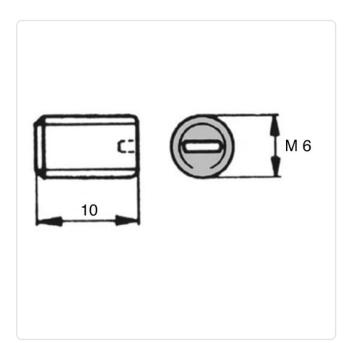
Color: Natural DIN/ISO: ISO4766 Drive Type: Slotted Flammability Class: UL94-V2 Length [mm]: 10 Material: PA 6.6 Material Group: Plastic Point Type: Flat Point Thread Size: M6 0.21g
