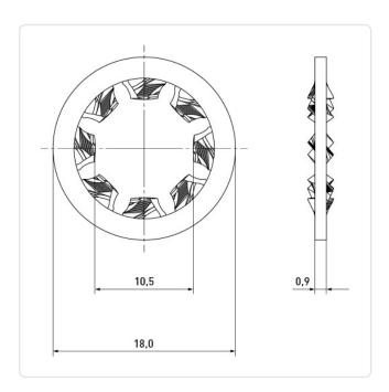
DIN/ISO: **DIN6798I** Finish: Plain For Thread Size: M10 0.9 Height [mm]: Inner Diameter [mm]: 10.5
