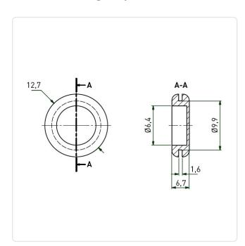
Color: Black Height [mm]: 6.7 Inner Diameter [mm]: 6.4 PVC Material: Material Group: **Plastic** Max. Panel Thickness [mm]: 1.6
