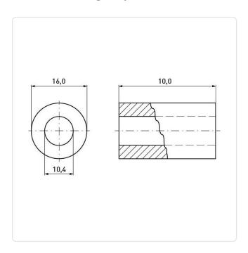
Color: Natural Flammability Class: UL94-HB For Thread Size: M10 Inner Diameter [mm]: 10.4 Length [mm]: 10
