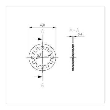
DIN/ISO: **DIN6797I** Finish: Plain For Thread Size: М3 0.4 Height [mm]: Inner Diameter [mm]: 3.2
