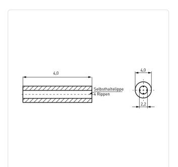
Color: Black Flammability Class: UL94-V2 For Thread Size: M2 Inner Diameter [mm]: 2.2 Length [mm]:
