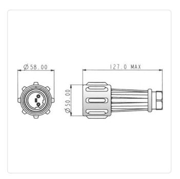
Amperage [A]: 32 Color: Black Protection Code: IP68 Weight: 135.2g
