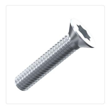
Torx T6 Actuator Size: DIN/ISO: ISO14581 Drive Type: **TORX** Plain Finish: Head Diameter [mm]: 3.8 Head Height [mm]: 1.2
