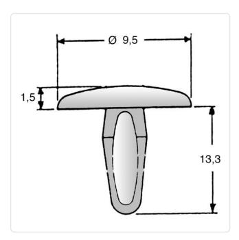
Color: Natural Flammability Class: UL94-V2 Head Diameter [mm]: 9.5 PA 6.6 Material: Material Group: **Plastic**
