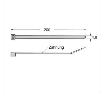
Bundle Diameter [mm]:21,0-50,0Color:NaturalFlammability Class:UL94-V2Length [mm]:200Material:Polyamide 6.0 25% GFWidth [mm]:4.8Weight:1.24gConformities:Reach
