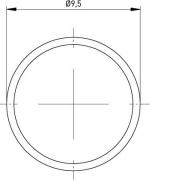
Bumper Design: Semicircular Color: Transparent Diameter [mm]: 9.5 Flammability Class: UL94-HB Height [mm]: 3.8 Material: PUR - Polyurethane Weight: 0.25g Conformities: Reach RoHS **SVHC**
