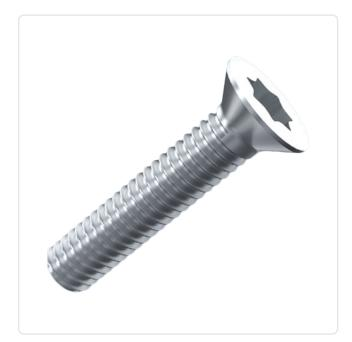
Torx T10 Actuator Size: DIN/ISO: ISO14581 Drive Type: **TORX** Plain Finish: Head Diameter [mm]: 5.5 Head Height [mm]: 1.65
