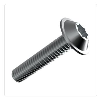
Actuator Size: Torx T20 DIN/ISO: ISO7380-2 Drive Type: **TORX** Plain Finish: Head Diameter [mm]: 9.4 Head Height [mm]: 2.2
