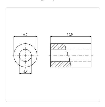
Finish: Plain For Thread Size: M4 Inner Diameter [mm]: 4.4 Length [mm]: 10
