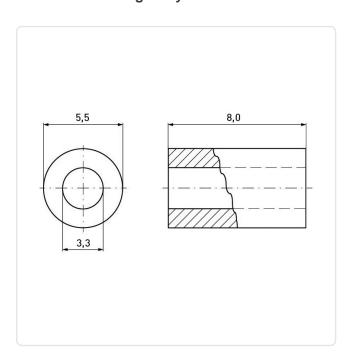
Finish: Plain For Thread Size: M3 Inner Diameter [mm]: 3.3 Length [mm]:
