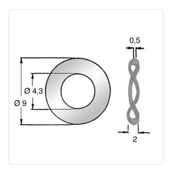
DIN/ISO: DIN137B Finish: Plain For Thread Size: M4 0.5 Height [mm]: Inner Diameter [mm]: 4.3
