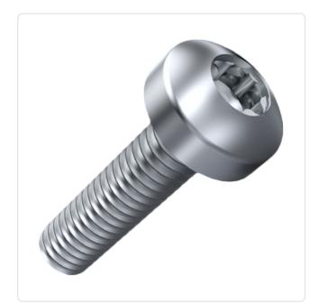
Torx T6 Actuator Size: DIN/ISO: ISO14583 Drive Type: **TORX** Plain Finish: Head Diameter [mm]: 4 Head Height [mm]: 1.6
