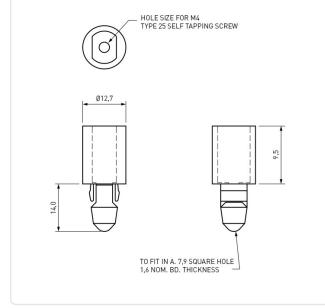
Color: Natural Flammability Class: UL94-V2 Length [mm]: 9.5 Polycarbonate Material: Material Group: Plastic Panel Hole Ø [mm]: 7.9 Panel Thickness [mm]: 1,6 Weight: 1.4g Conformities: Reach RoHS SVHC
