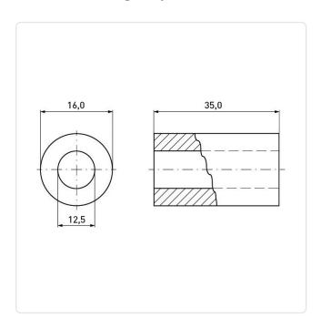
Color: Black Flammability Class: UL94-HB For Thread Size: M12 Inner Diameter [mm]: 12.5 Length [mm]: 35
