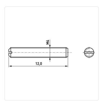
Color: Natural DIN/ISO: ISO4766 Drive Type: Slotted Flammability Class: UL94-V2 Length [mm]: 12 Material: PA 6.6 Material Group: Plastic Point Type: Flat Point Thread Size: M4
