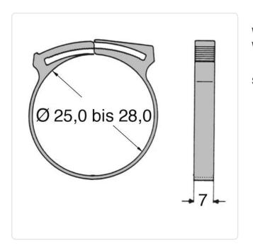
Color: Black Flammability Class: UL94-V2 PA 6.6 Material: Panel Thickness Range [mm]: 25,0-28,0
