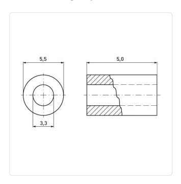
Finish: Plain For Thread Size: М3 Inner Diameter [mm]: 3.3 Length [mm]:
