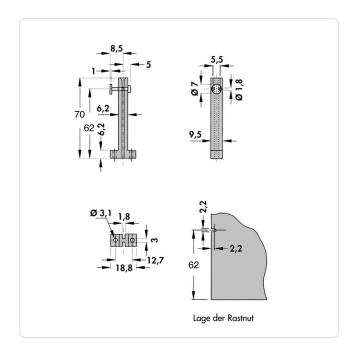
Color: Gray Dist. Mounting Holes [mm]: 12.7 Flammability Class: UL94-V0 70
