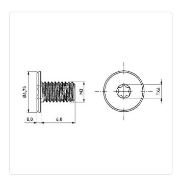
Torx T6 Actuator Size: Drive Type: **TORX** Finish: Plain Head Diameter [mm]: 6.75 Head Height [mm]: 8.0
