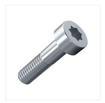
Actuator Size: Torx T10 DIN/ISO: ISO14580 Drive Type: **TORX** Plain Finish: Head Diameter [mm]: 5.5 Head Height [mm]: 2.4
