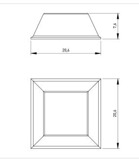
Bumper Design: Square, Tapered Color: Transparent Diameter [mm]: 20.6 Flammability Class: UL94-HB Height [mm]: 7.6 Material: PUR - Polyurethane Weight: 2.56g Conformities: Reach SVHC
