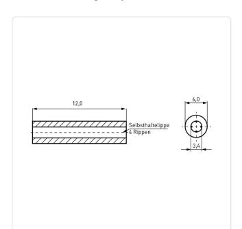
Color: Black Flammability Class: UL94-V2 For Thread Size: M3 Inner Diameter [mm]: 3.4
