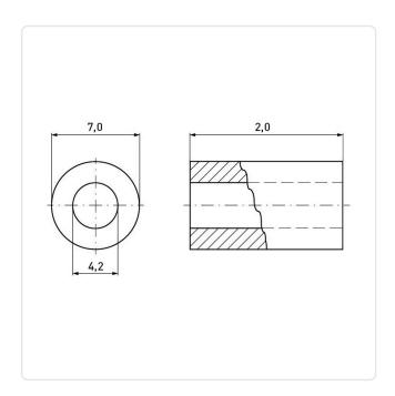
Finish: Plain For Thread Size: M4 Inner Diameter [mm]: 4.2 Length [mm]:
