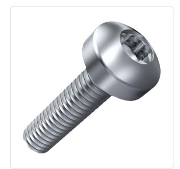
Actuator Size: Torx T10 Drive Type: **TORX** Finish: Plain Head Diameter [mm]: 5.4 Head Height [mm]: 1.9
