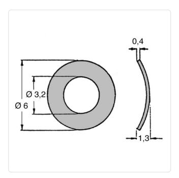
DIN/ISO: DIN137A Finish: Plain For Thread Size: M3 0.4 Height [mm]: Inner Diameter [mm]: 3.2
