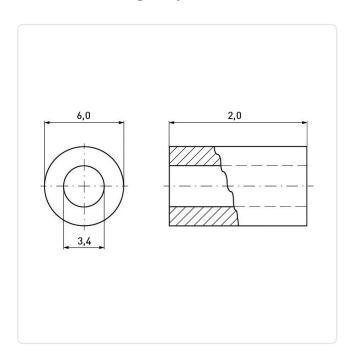
Color: Natural Flammability Class: UL94-V2 For Thread Size: М3
