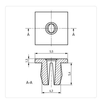
AF / OD [mm]: 5.6 Color: Natural Head Height [mm]: 1.3 Length [mm]: 5.6 Material: PA 6.6 Material Group: Plastic Panel Cutout [mm]: 4.3x4.3 Panel Thickness [mm]: 0,8-2,0 Thread Diameter [mm]: Ø 2.9
