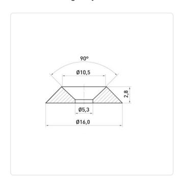
Finish: Plain For Thread Size: M5 Height [mm]: 2.8 Inner Diameter [mm]: 5.3
