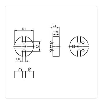
Flammability Class: UL94-V0 Inner Diameter [mm]: 2.5
