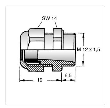
AF / OD [mm]: 14 Brass Material: Material Group: **Brass** Mounting Hole [mm]: 12.5 Panel Thickness Range [mm]: 3,0-6,5 Protection Code: IP68 Thread Size: M12 Weight: 10.68g Conformities:
