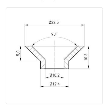
Inner Diameter [mm]: 10.2 Lug Diameter [mm]: 12.4 Material: PA<sub>6</sub> Material Group: Plastic
